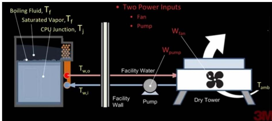
Open Bath Immersion Cooling System Schematic by 3M™
